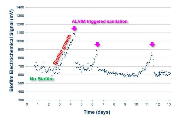
This approach allowed for a **reduction of more than 90% in the total amount of chlorine used in the plant, without any loss of efficiency**. At the same time, the ALVIM System allowed to check the effectiveness of the biocide. Taking into account that a large desalination plant can spend up to 1.5 million \$ per year in biocides, the use of the ALVIM Biofilm Monitoring System can provide great savings.
